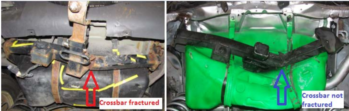
Figure 26 - Left: Real-world crash cross-member fracture, Right: Reconstruction deformation, no cross-member fracture
