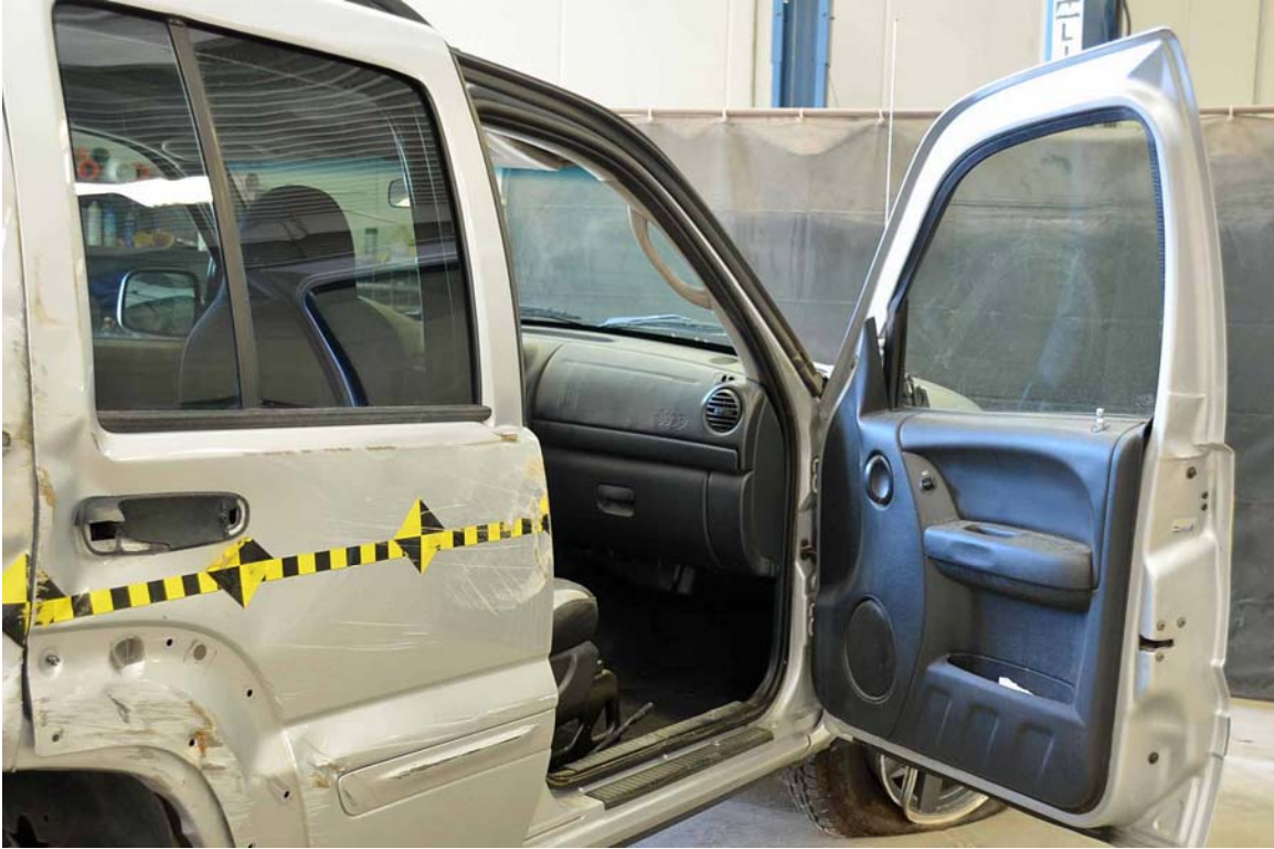
FIGURE 149. Post-Test Door Opening
