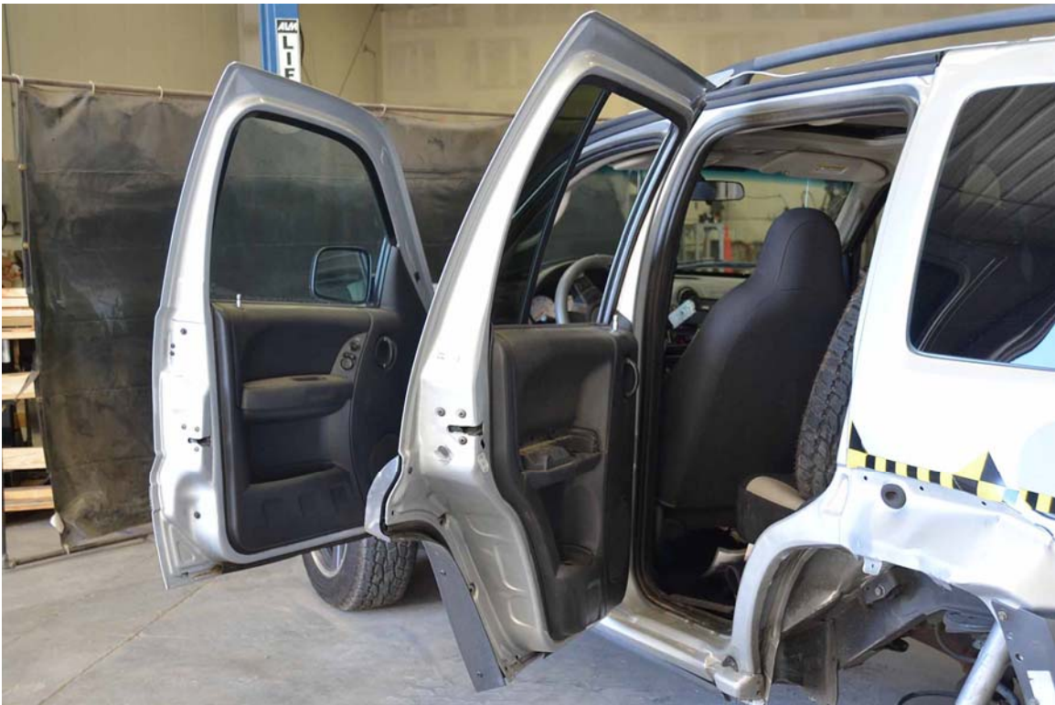
FIGURE 148. Post-Test Door Opening
