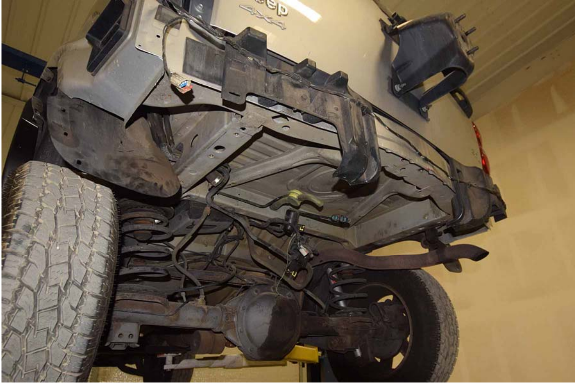
FIGURE 39. 2003 Jeep Liberty with Fuel Tank Removed
