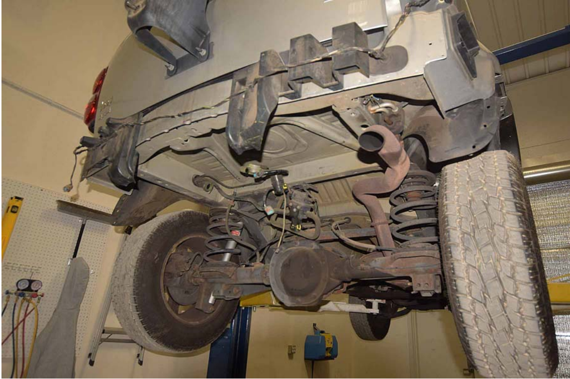
FIGURE 41. 2003 Jeep Liberty with Fuel Tank Removed
