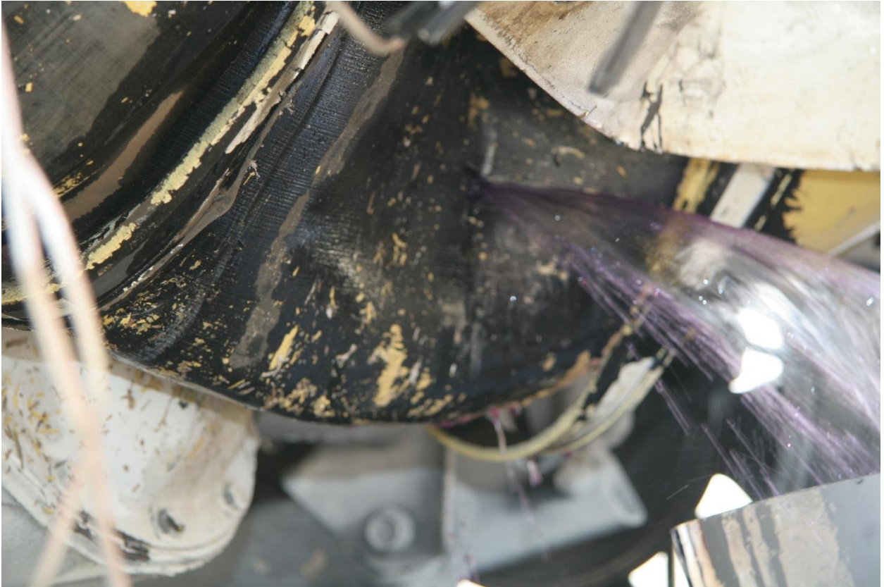
Exhibit D –Leak from Ruptured Grand Cherokee Fuel Tank in 40-mph Impact
