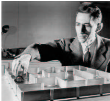
Figure 5: Shannon with Theseus, a mechanical mouse that was some of the earliest work in machine learning.
