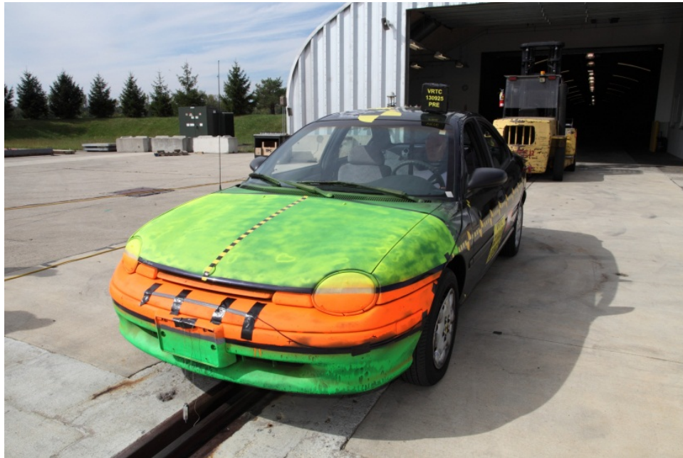
Figure 5 - 1997 Plymouth Neon bullet vehicle with painted regions
