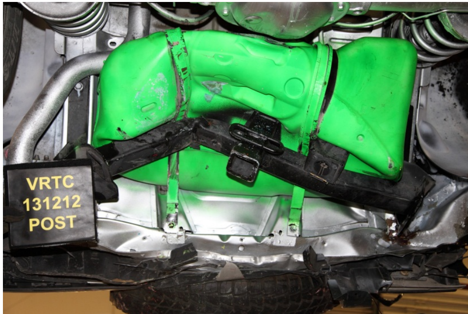
Figure 29 - Test #8 Post-test target vehicle fuel tank close-up view
