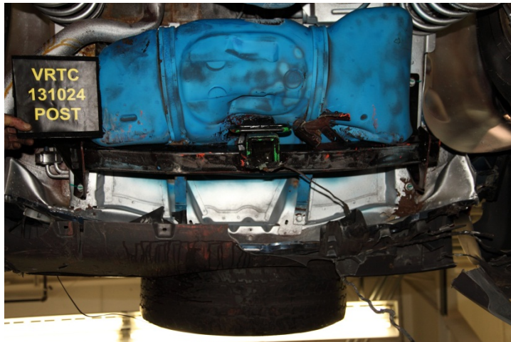
Figure 10 – Test #2 Post-test target vehicle fuel tank close-up view with hitch-receiver
