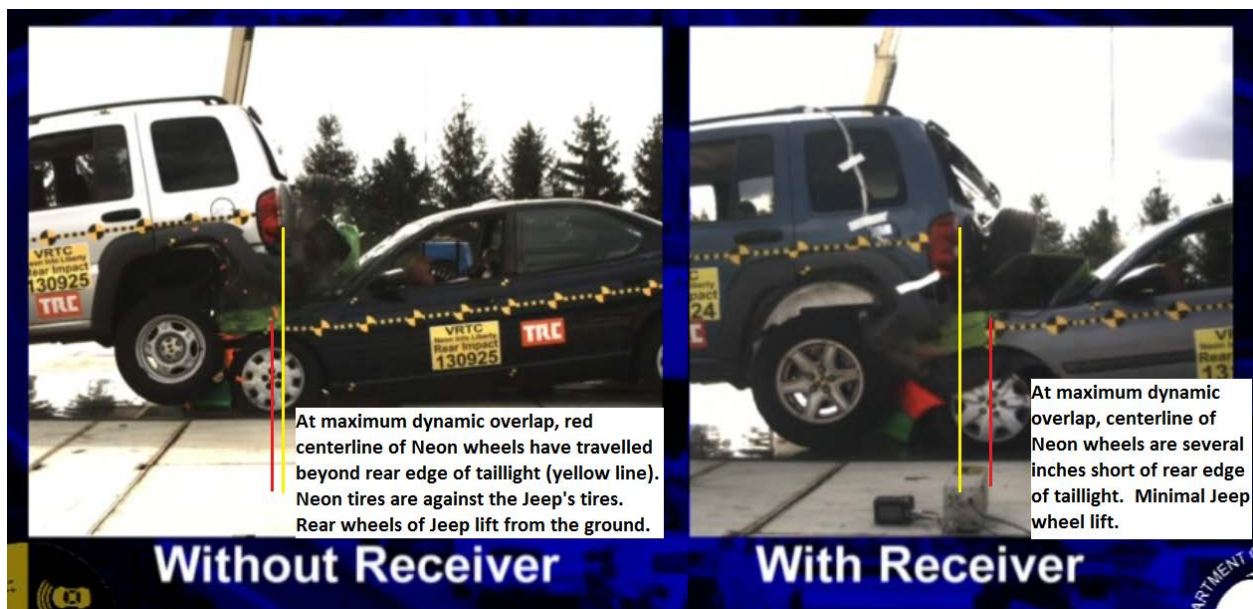
Figure 6 - Difference in dynamic overlap of Neon and Jeep Liberty
