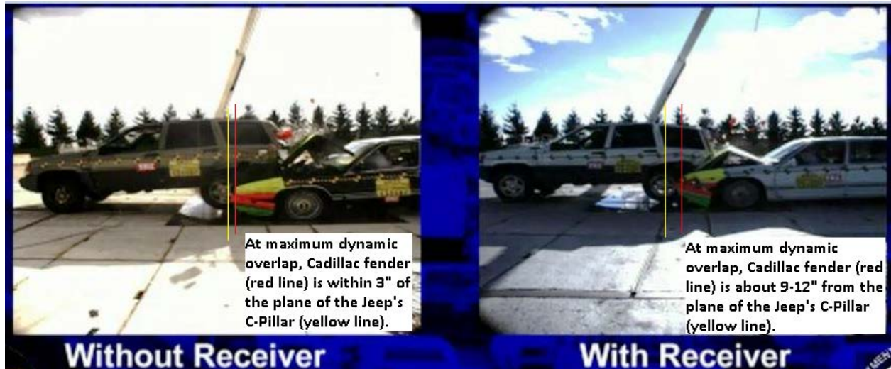
Figure 14- Dynamic overlap between Cadillac and Jeep Grand Cherokee without and with a hitch-receiver
