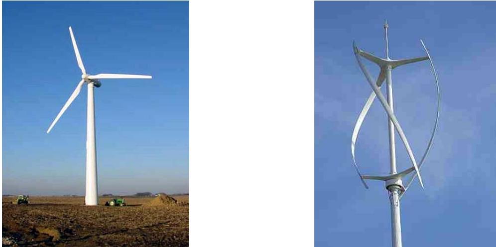
Figure 30 (a) A horizontal axis wind turbine; (b) A vertical axis turbine
