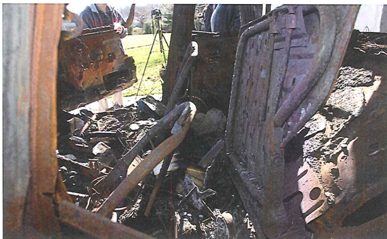
Figure 1. Photograph showing the deformation of the first and second row seatbacks.
