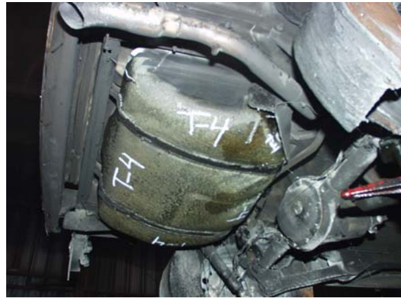
Figure 16. "Square" tank after fire test.
