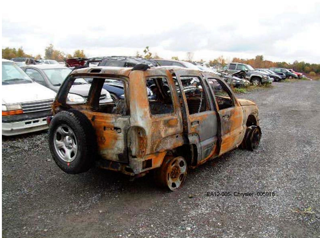
Figure 3 - Post-Crash photograph of 2004 Jeep Liberty Struck from behind by a Plymouth Neon.
