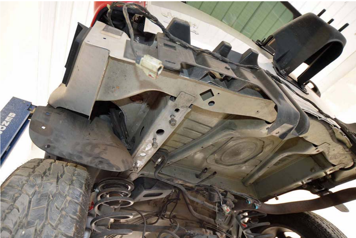
FIGURE 24. 2003 Jeep Liberty Fuel Tank Removed
