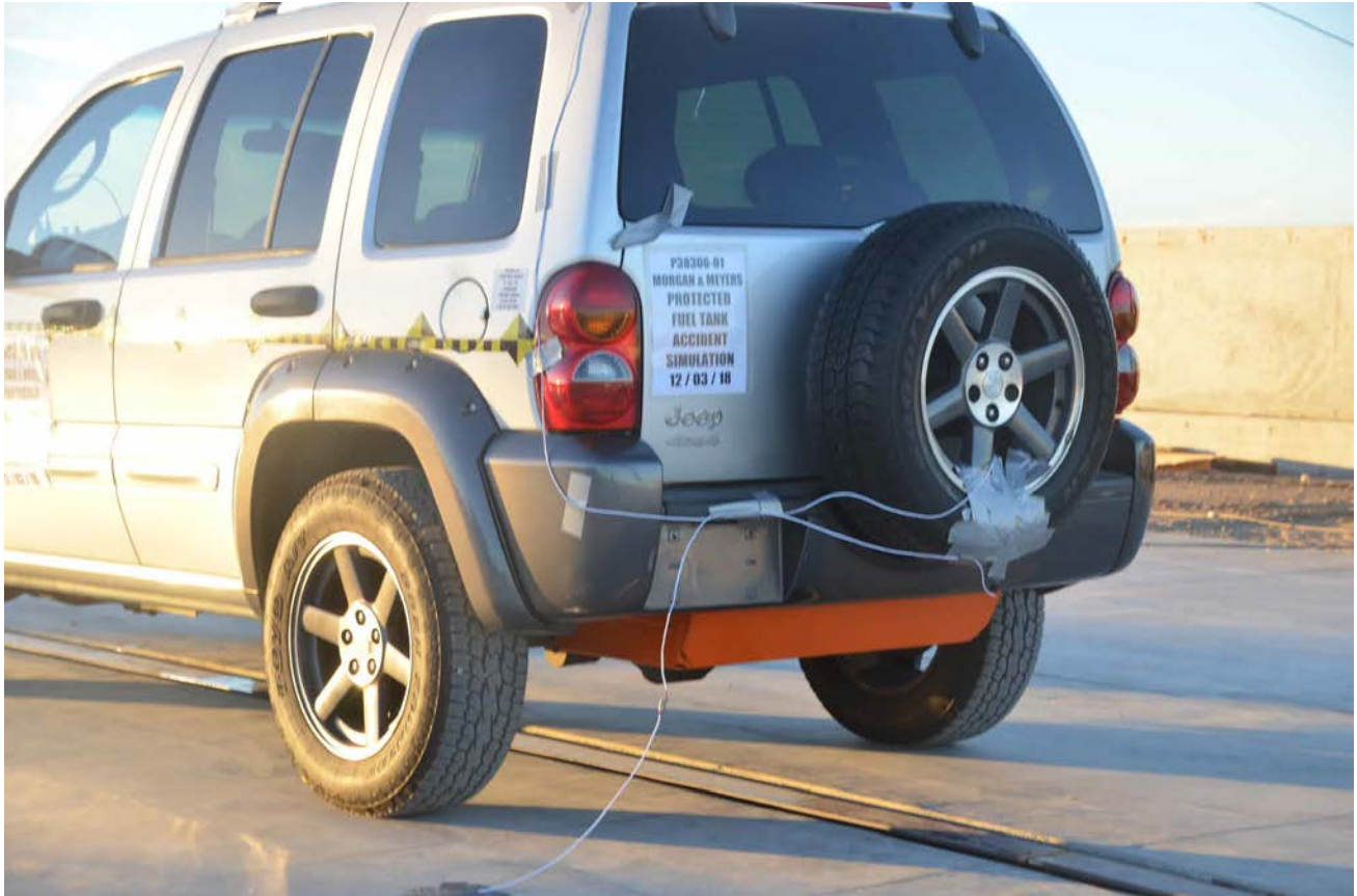
Pictorial presentation/review of the mock-up, fabrication/construction, and installation process of the FTEP onto a typical Jeep Liberty KJ
