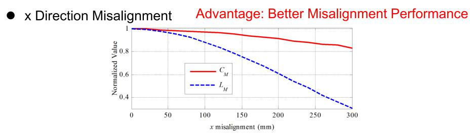
C<sub>M</sub> remains 84.2% of the well-aligned value, L<sub>M</sub> remains 30% of the wellaligned value
