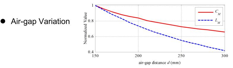
C<sub>M</sub> remains 66.5% of the well-aligned value, L<sub>M</sub> remains 41% of the well-aligned value
