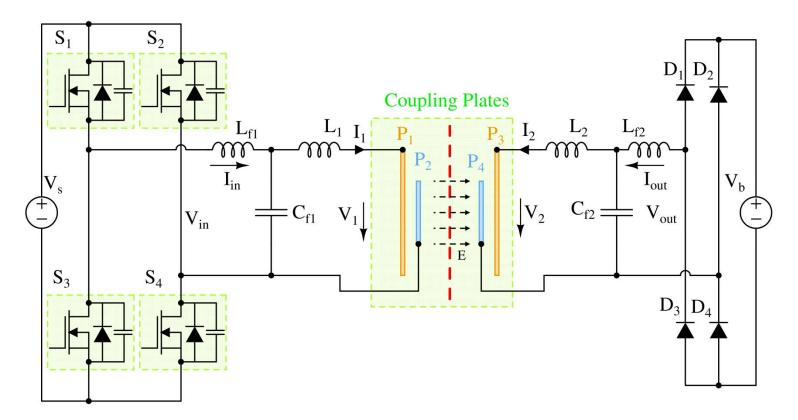
Compensation topology is simplified and The LCL compensation circuit is used to resonate with the plates, instead of the LCLC topology
