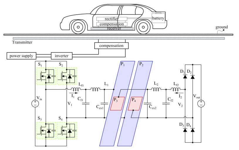
Reduce system cost using metal plates as capacitive couplers
