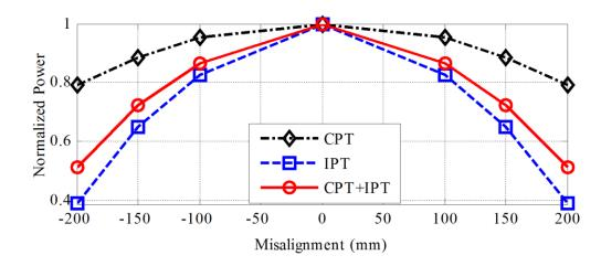
Output power drops to 1.35 kW at 200 mm misalignment (47.5% of wellaligned power)
