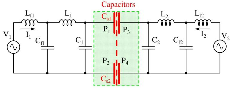
> At input inverter side,  $V_1$  and  $I_1$  are in phase
