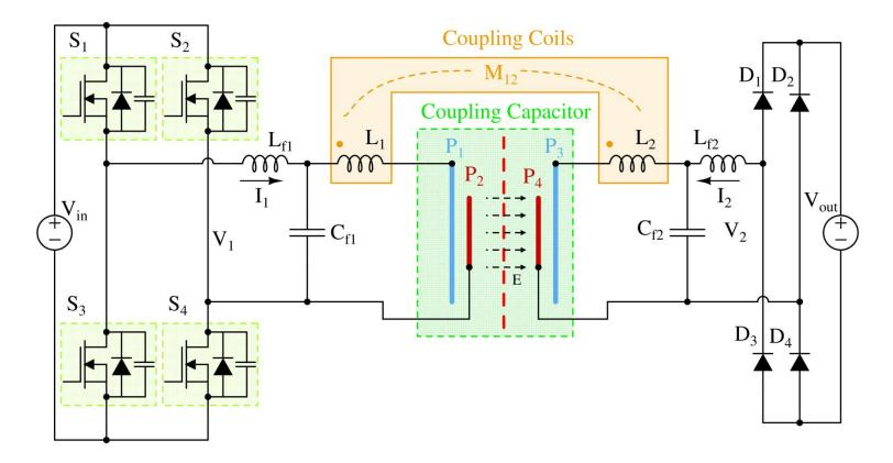
The two inductors L<sub>1</sub> are L<sub>2</sub> are inductively coupled
