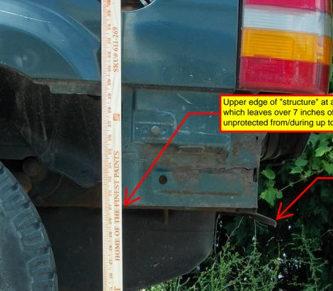
Upper edge of "structure" at approximately 21.25 inches, which leaves over 7 inches of unprotected fuel tank; unprotected from/during up to 270 degrees of impact angles.
