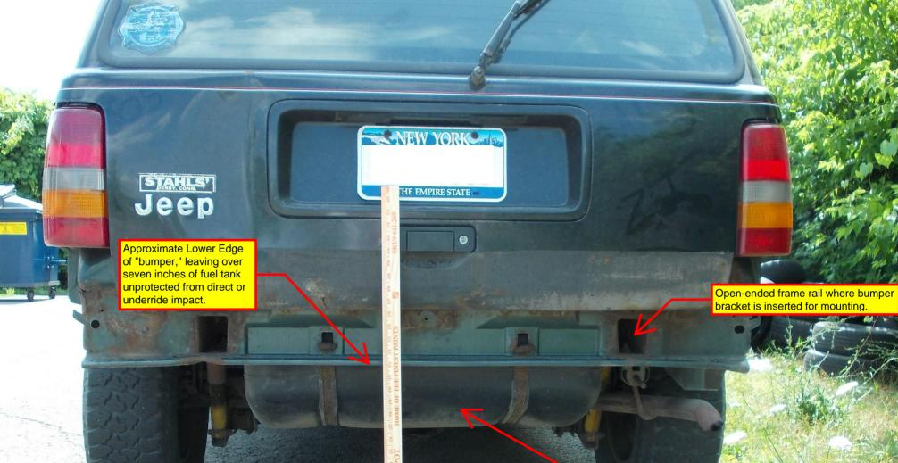
Unprotected Polyethylene fuel tank
