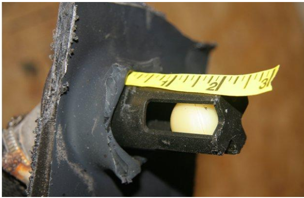
Picture 2 – Ineffective Grand Cherokee Check Valve
