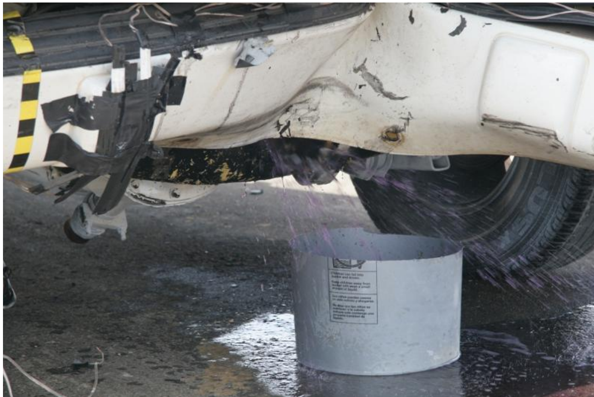
Picture 13 – Fuel Leakage from Fuel Tank
