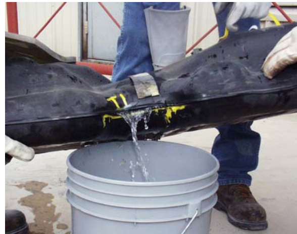
Figure 17. Seasoned “Long” Tank Post Drop Test
