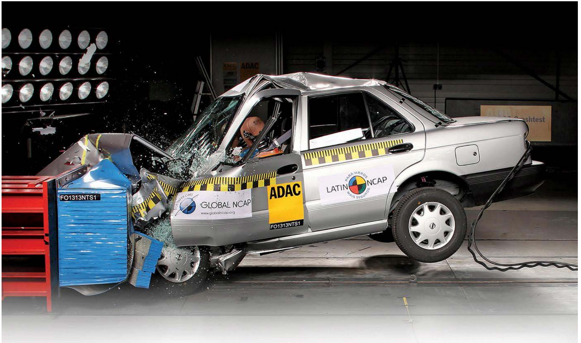
In Latin NCAP's crash testing, the popular Nissan Tsuru, based on an early-1990s Sentra, got zero stars. Airbags aren't available. PRINTED FROM: http://www.autonews.com/apps/pbcs.dll/article?AID=/20160619/OEM11/306209954&template=print
