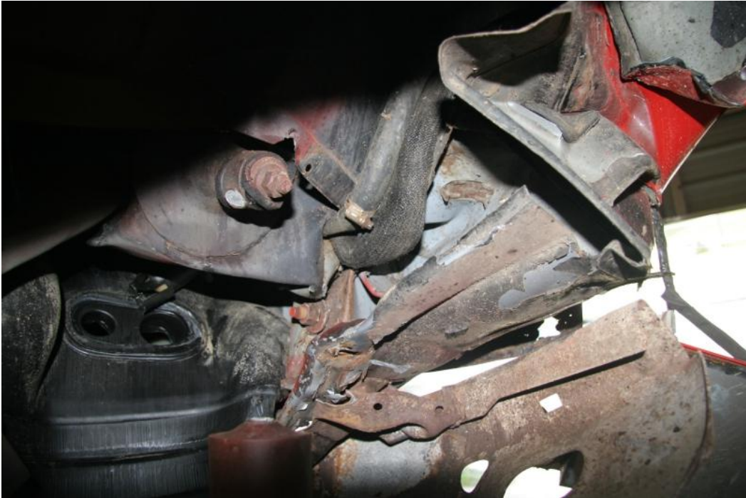
Picture 6 – Fuel Filler/Emission Control Line Plate Failure
