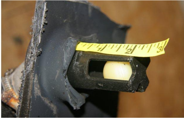
Picture 2 – Ineffective Grand Cherokee Check Valve
