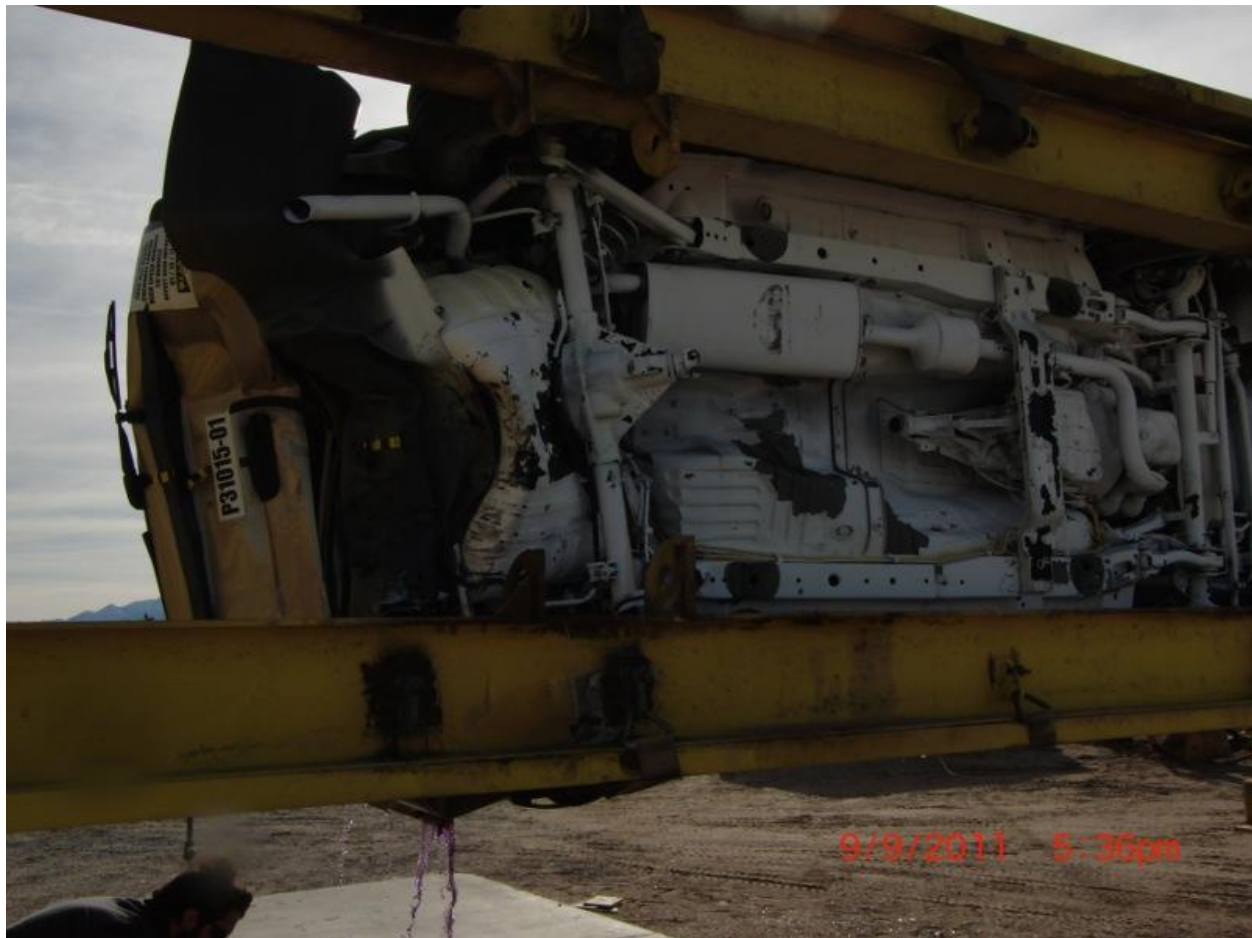
Picture 9 – Stoddard Fluid Leaking from Fuel Tank
