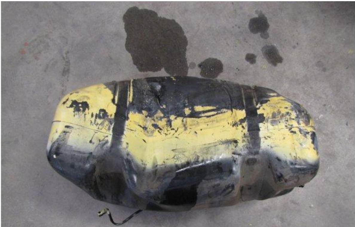
Picture 12 – 1996 Grand Cherokee Punctured Fuel Tank
