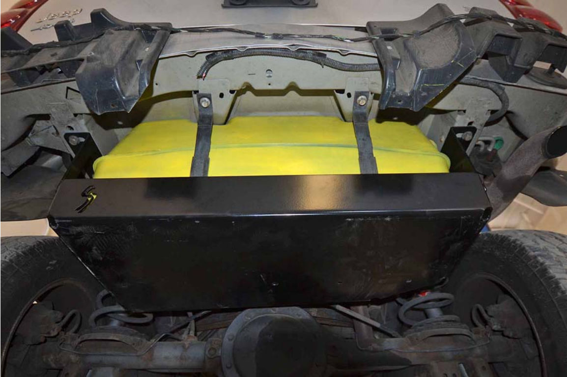
FIGURE 37. 2003 Jeep Liberty with SFK Manufacturing Model JP-4002 Skid Plate Installed
