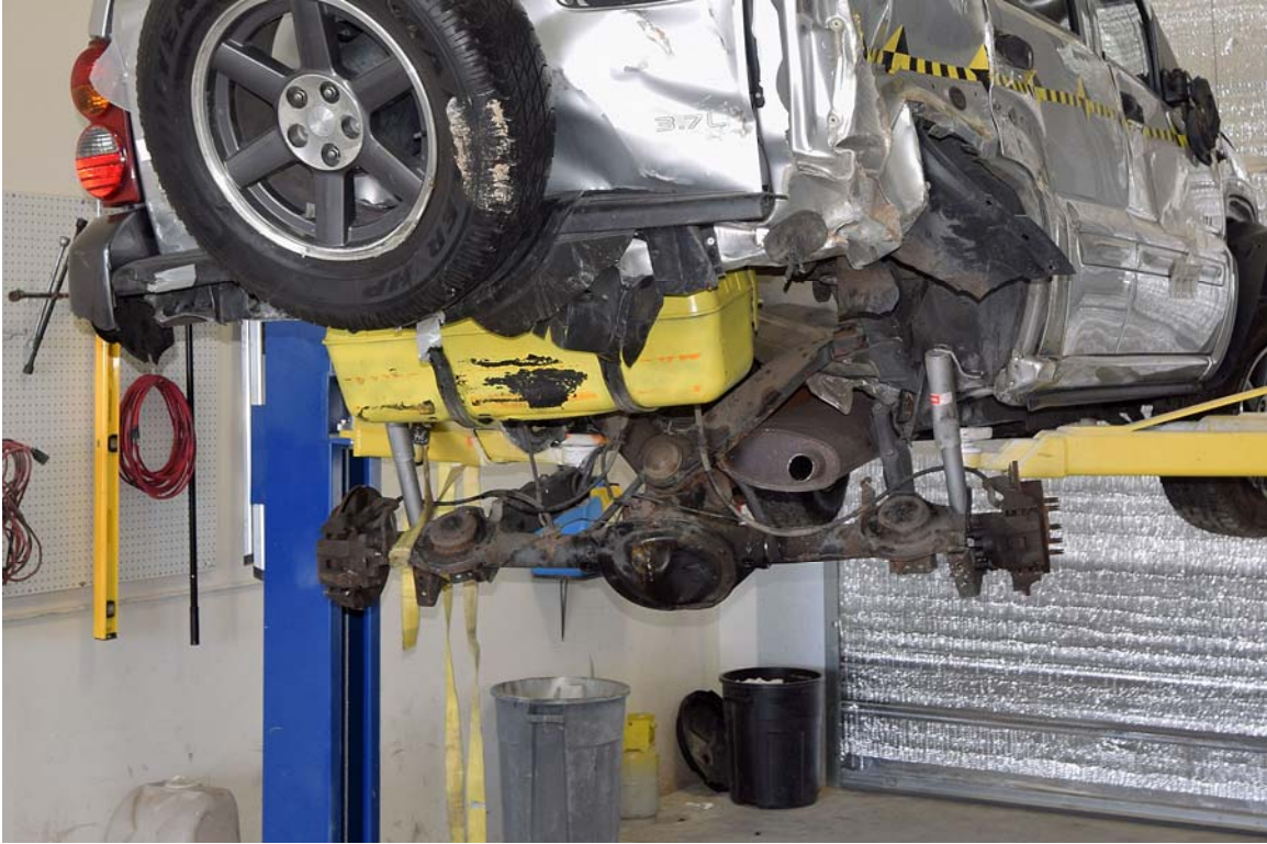
FIGURE 129. Post-Test Fuel Tank Inspection
