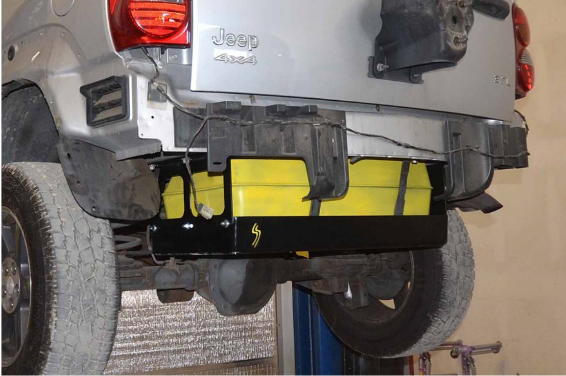
FIGURE 33. 2003 Jeep Liberty with SFK Manufacturing Model JP-4002 Skid Plate Installed
