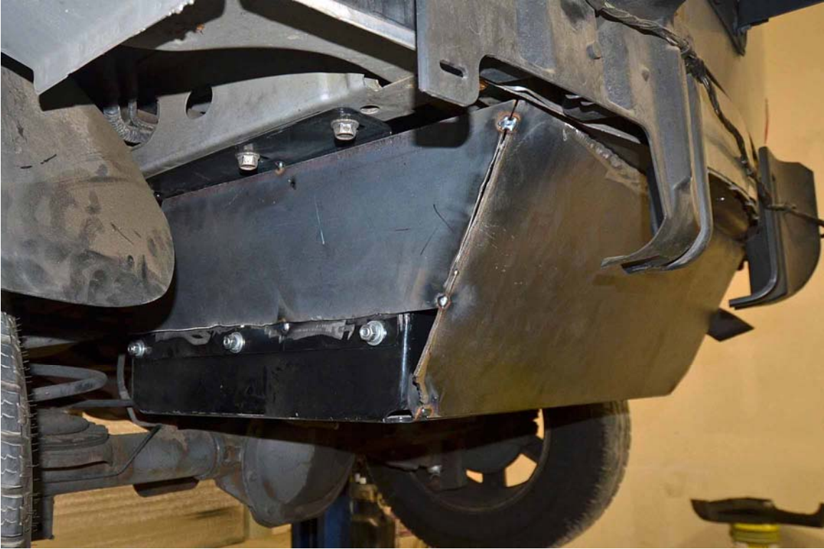
FIGURE 48. 2003 Jeep Liberty Fuel Tank Encapsulation Prototype Design Process
