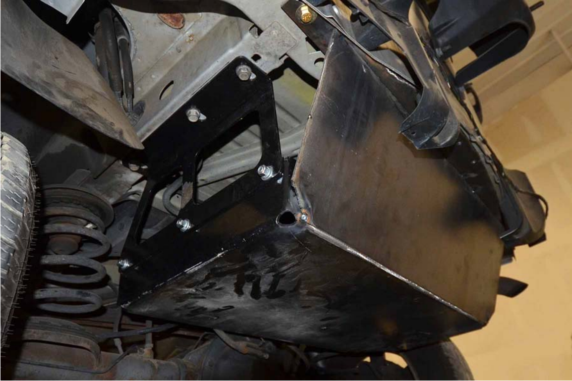
FIGURE 45. 2003 Jeep Liberty Fuel Tank Encapsulation Prototype Design Process
