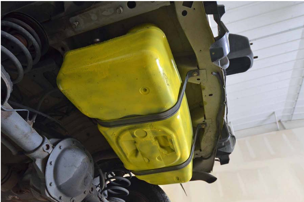
FIGURE 30. 2003 Jeep Liberty with Fuel Tank Reinstalled
