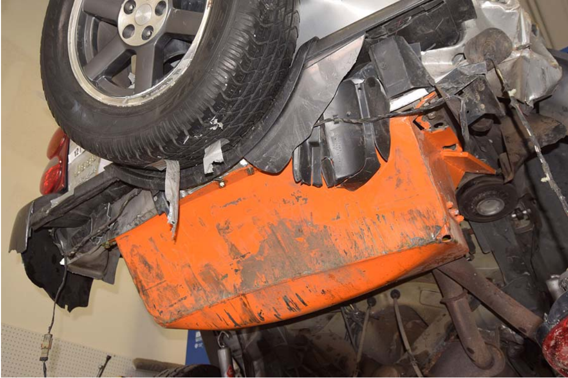
FIGURE 111. Post-Test Fuel Tank Inspection
