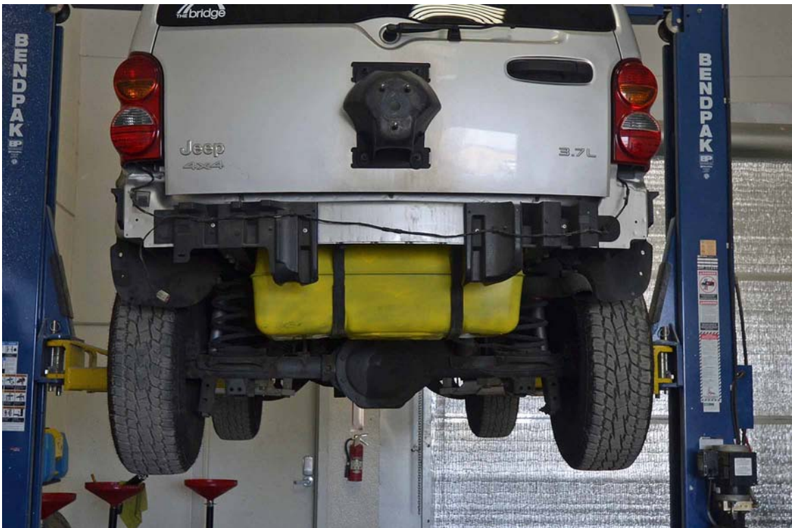
FIGURE 28. 2003 Jeep Liberty with Fuel Tank Reinstalled
