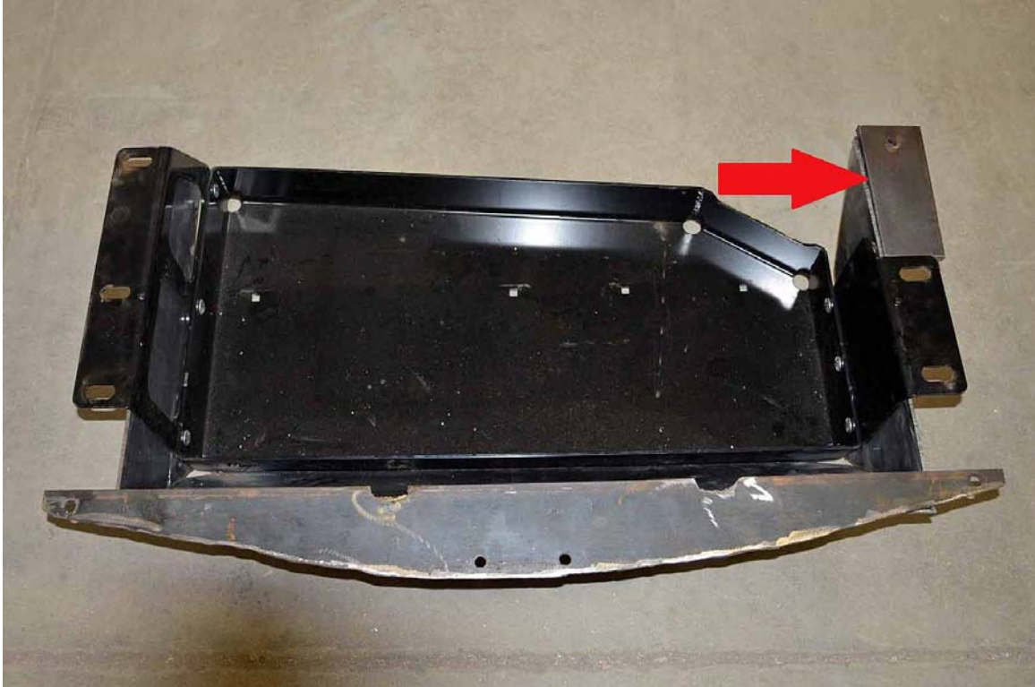
FIGURE 53. 2003 Jeep Liberty Fuel Tank Encapsulation Prototype Design Process Showing 1/2" Plate
