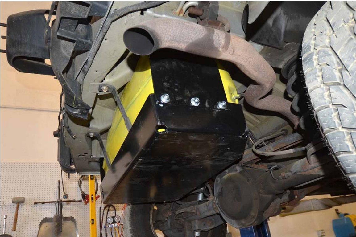
FIGURE 38. 2003 Jeep Liberty with SFK Manufacturing Model JP-4002 Skid Plate Installed
