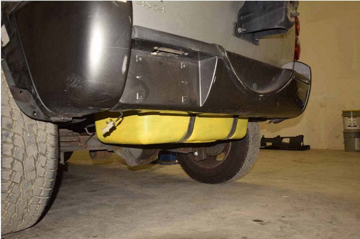
FIGURE 58. 2003 Jeep Liberty with Fuel Tank Re-Installed
