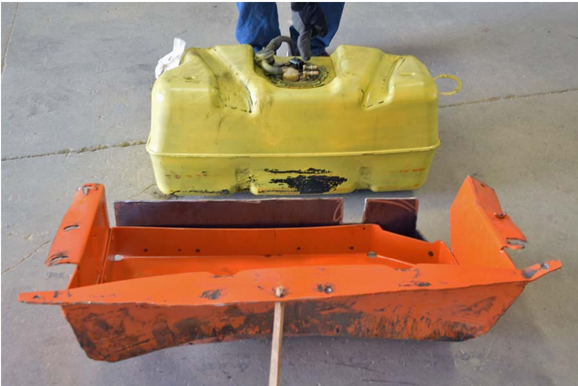
FIGURE 140. Post-Test Fuel Tank Inspection
