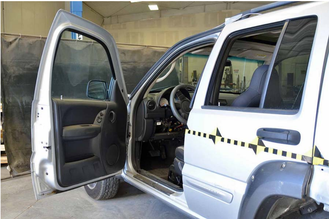
FIGURE 146. Post-Test Door Opening
