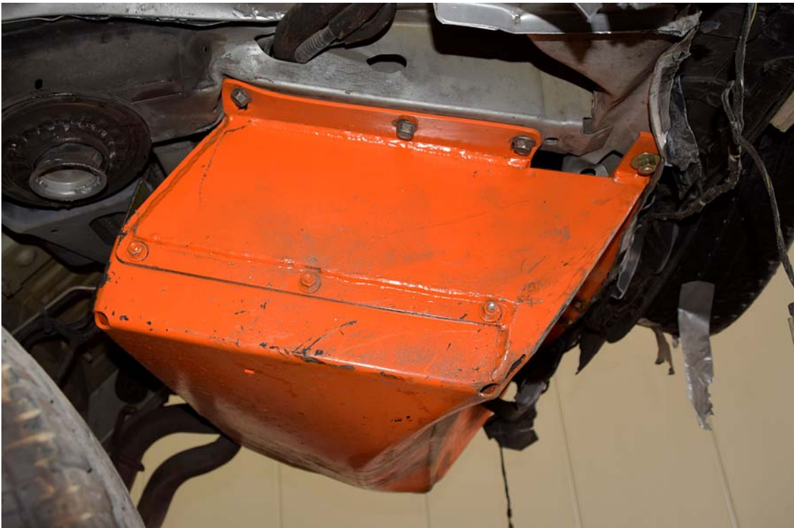
FIGURE 108. Post-Test Fuel Tank Inspection
