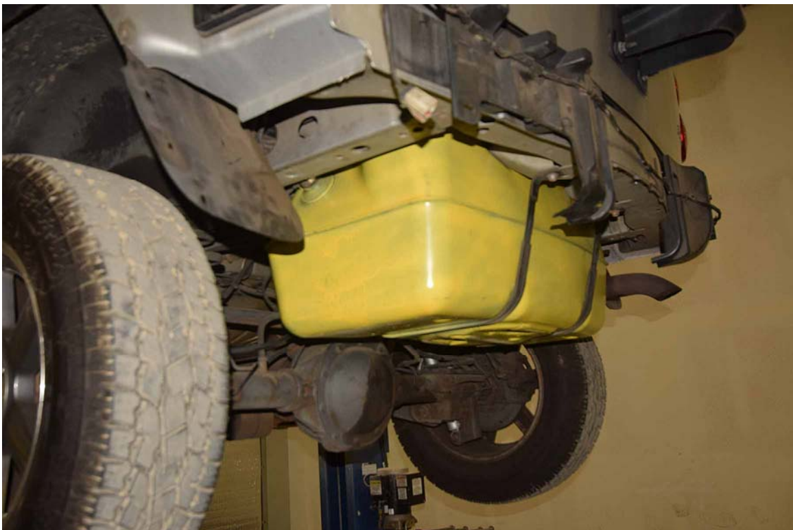
FIGURE 54. 2003 Jeep Liberty with Fuel Tank Re-Installed
