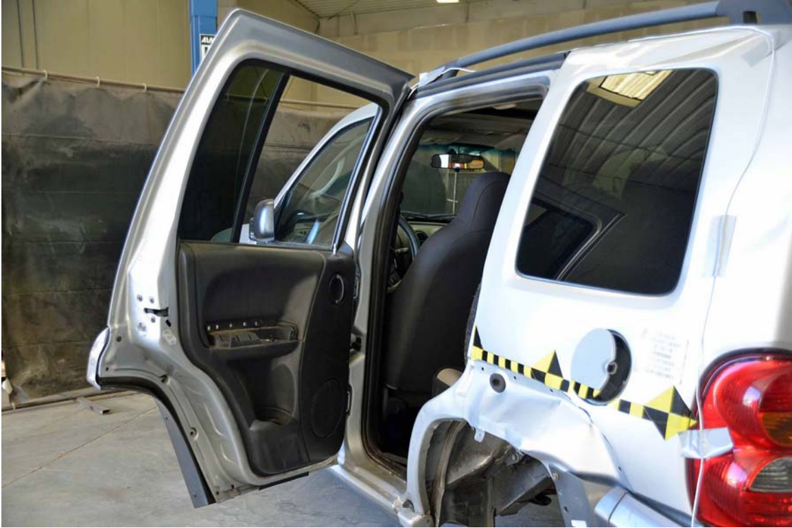
FIGURE 147. Post-Test Door Opening
