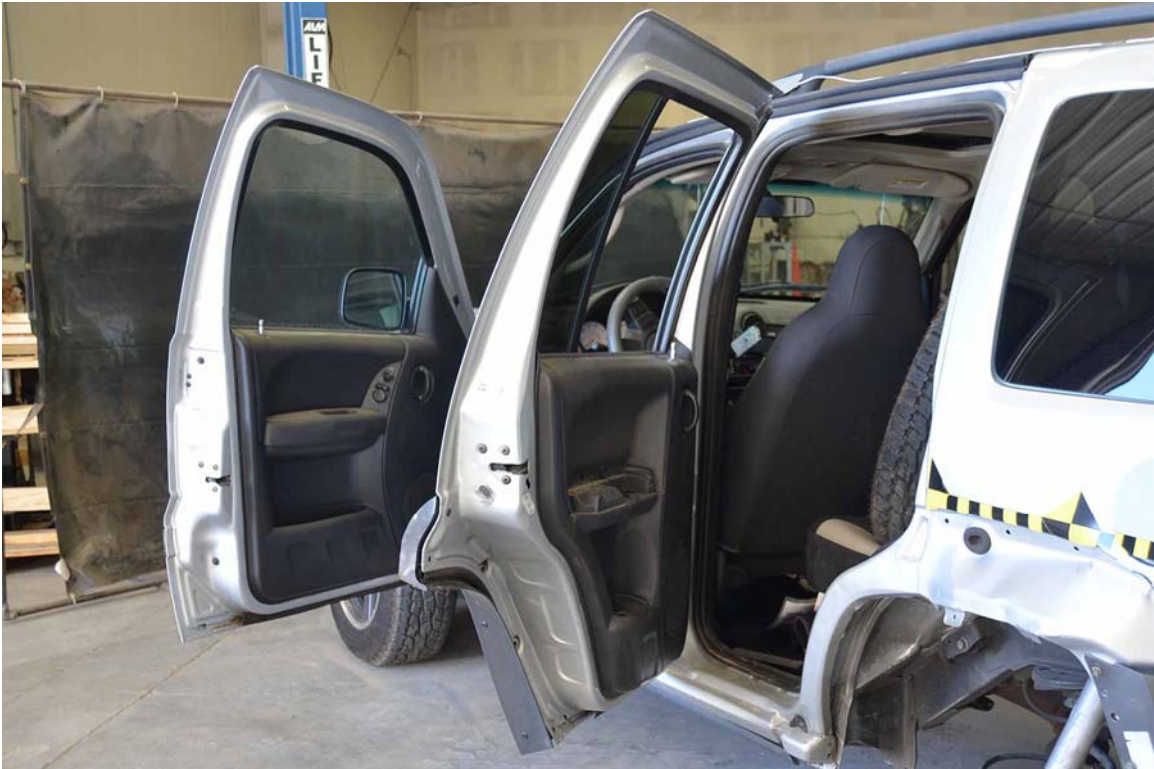
FIGURE 148. Post-Test Door Opening
