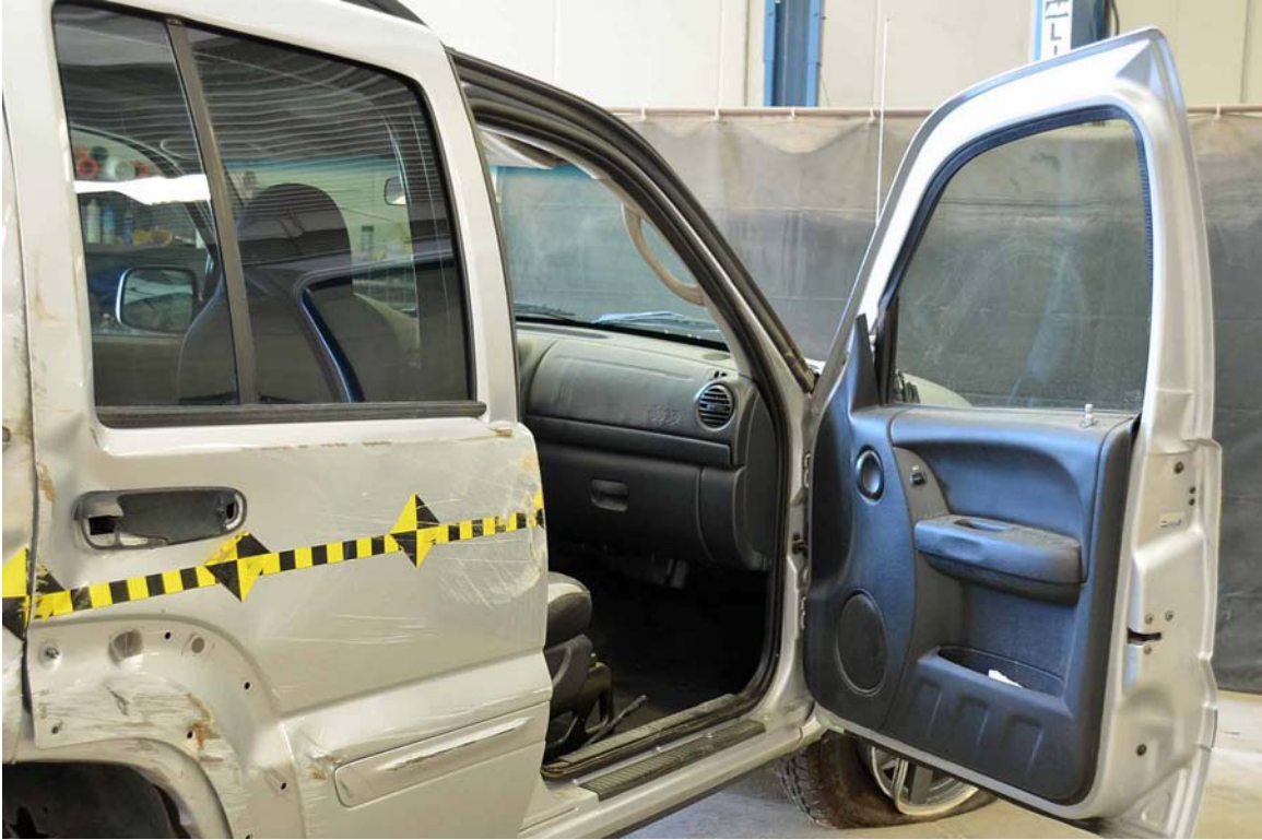
FIGURE 149. Post-Test Door Opening
