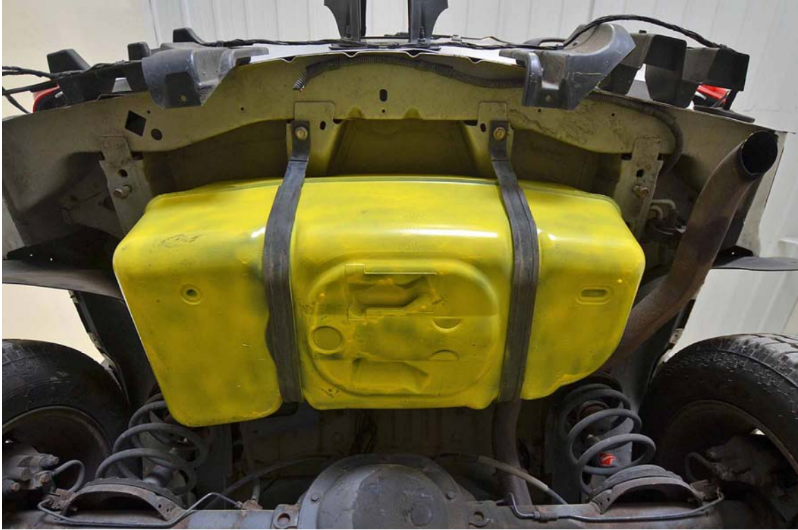
FIGURE 31. 2003 Jeep Liberty with Fuel Tank Reinstalled
