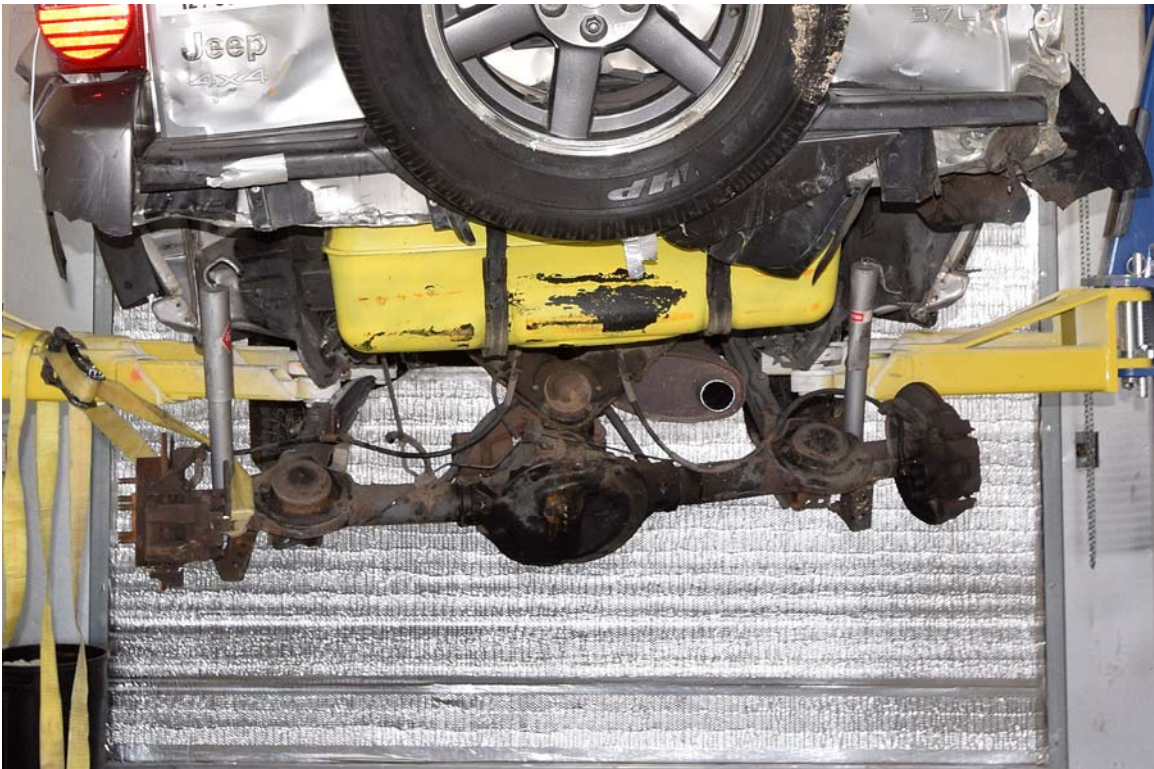
FIGURE 128. Post-Test Fuel Tank Inspection
