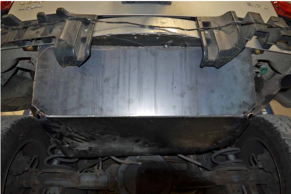
FIGURE 46. 2003 Jeep Liberty Fuel Tank Encapsulation Prototype Design Process
