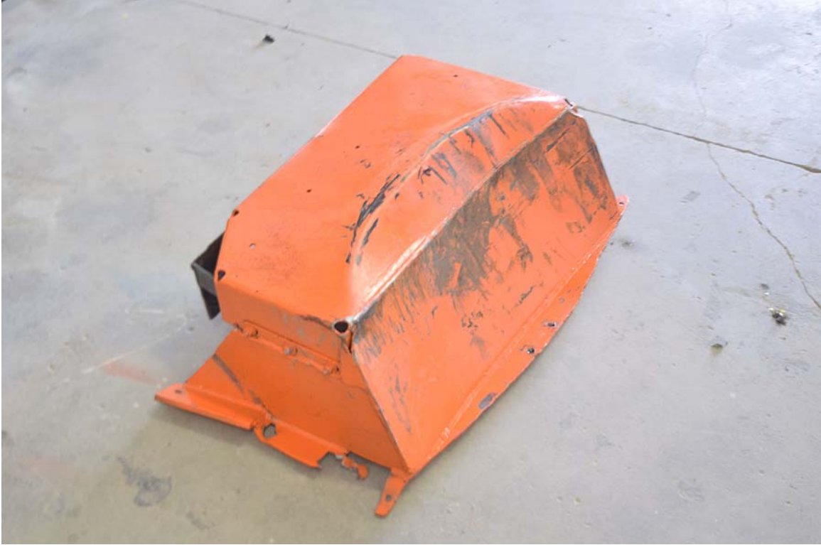
FIGURE 117. Post-Test Fuel Tank Inspection
