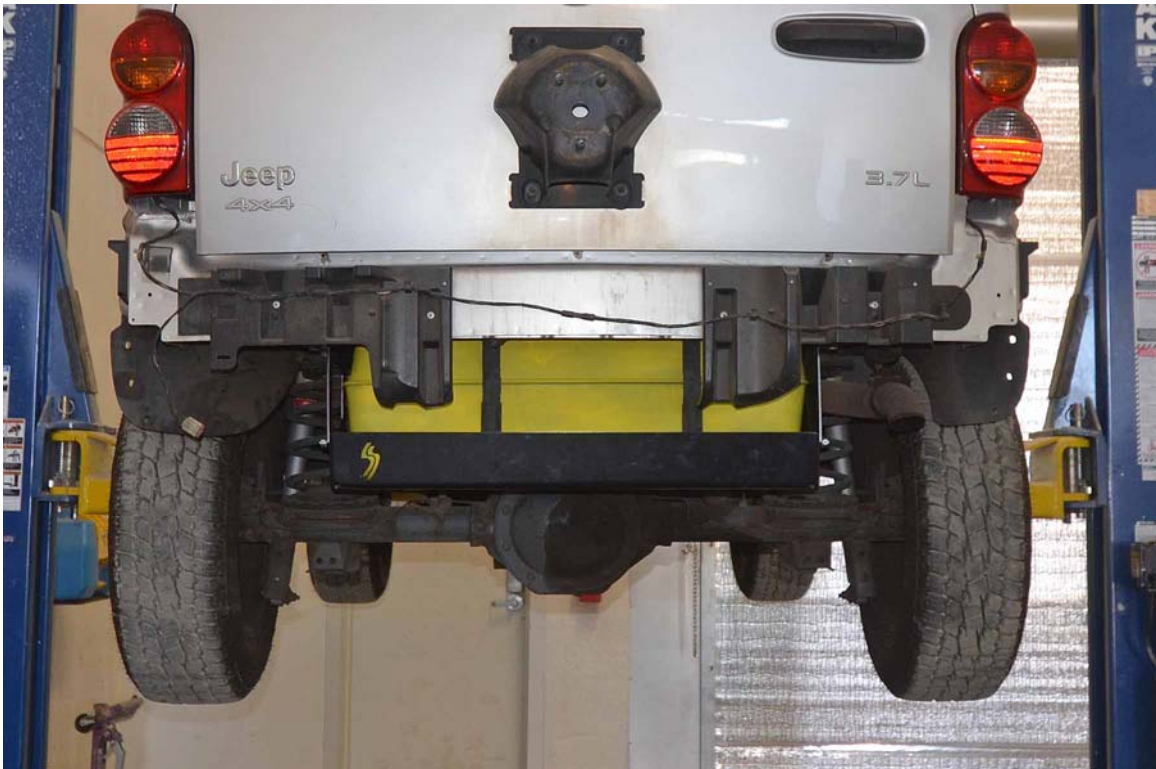
FIGURE 34. 2003 Jeep Liberty with SFK Manufacturing Model JP-4002 Skid Plate Installed
