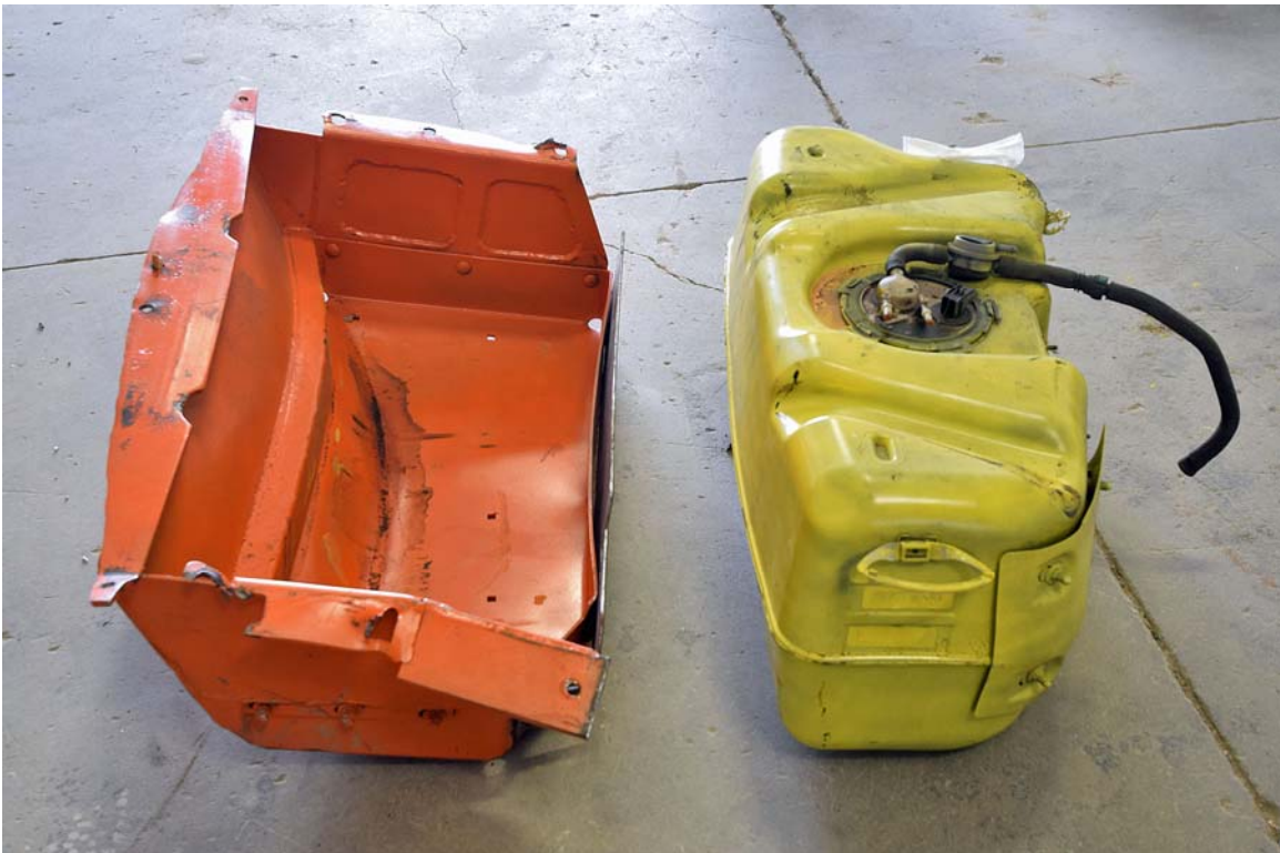
FIGURE 142. Post-Test Fuel Tank Inspection
