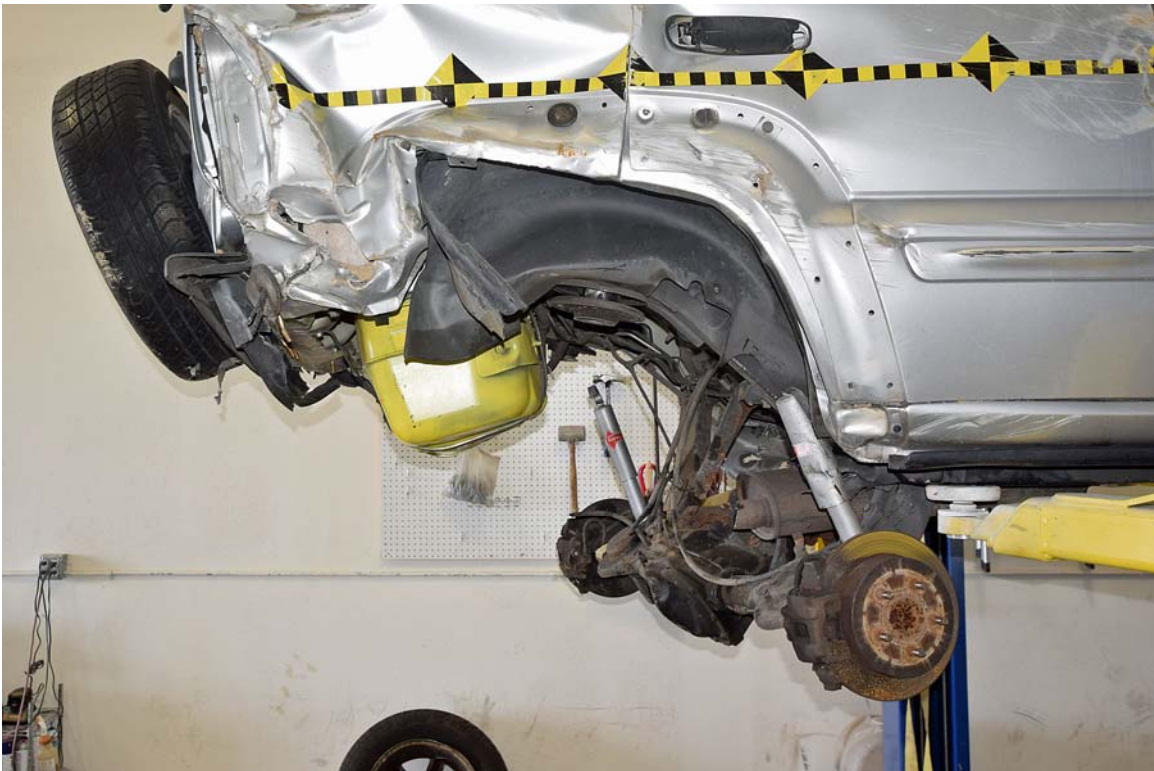
FIGURE 130. Post-Test Fuel Tank Inspection
