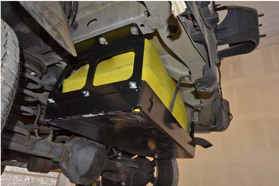
FIGURE 36. 2003 Jeep Liberty with SFK Manufacturing Model JP-4002 Skid Plate Installed
