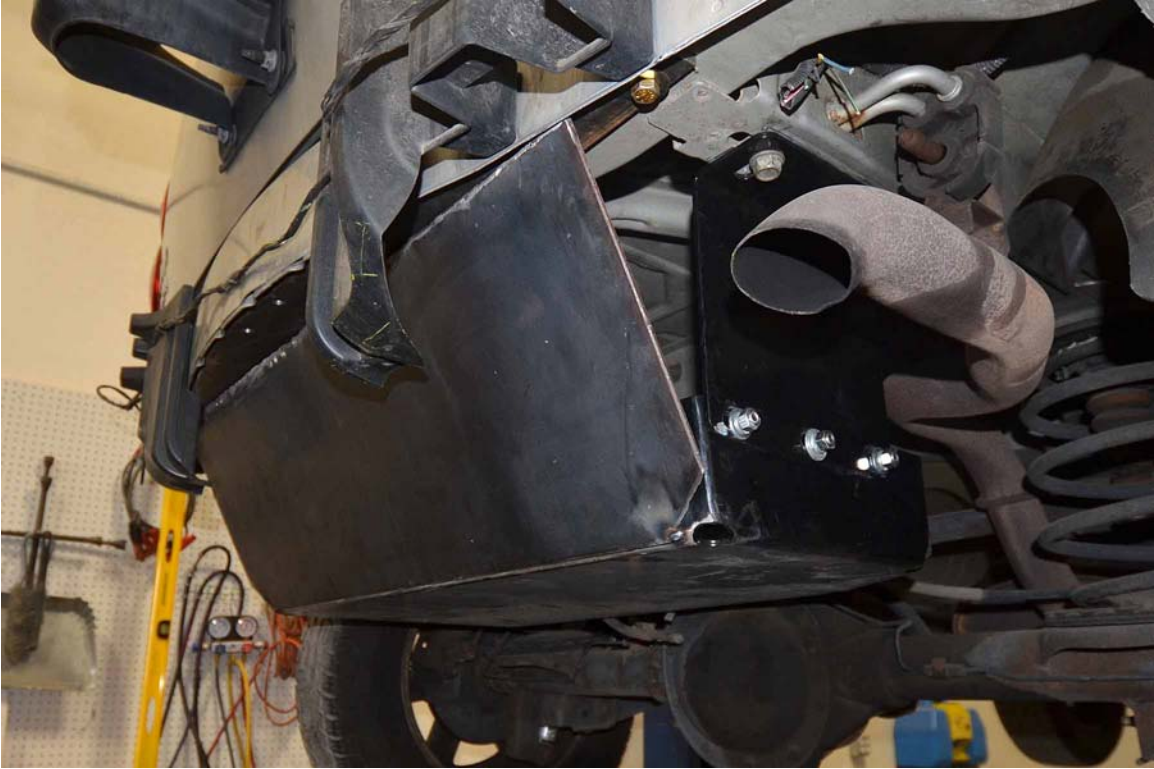
FIGURE 47. 2003 Jeep Liberty Fuel Tank Encapsulation Prototype Design Process
