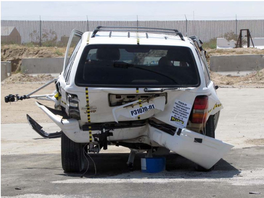
FIGURE 34. Post-Test Target Vehicle, Rear
