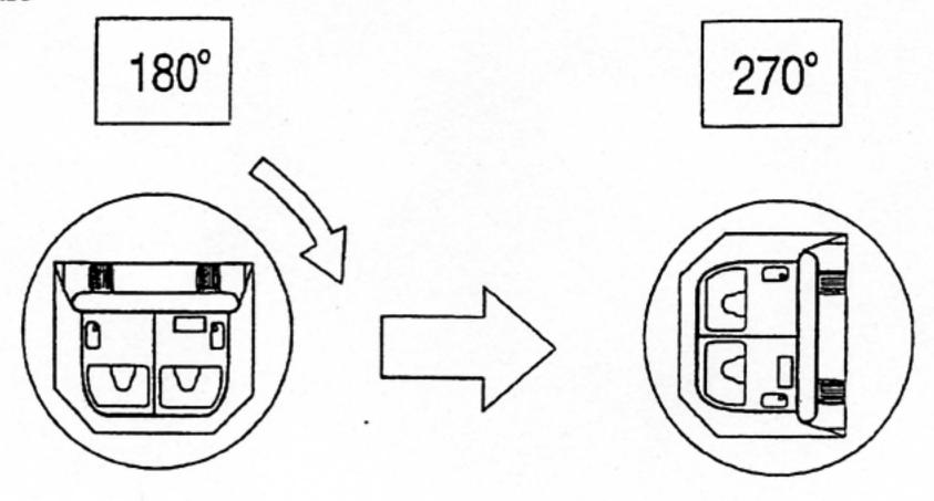
Static rollover machine rotation time information: (specified range is 1-3 minutes)
