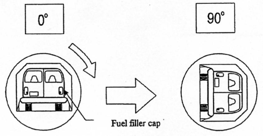
Static rollover machine rotation time information: (specified range is 1-3 minutes)
