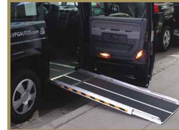
The ramp is positioned on the side of the vehicle allowing passengers to enter and exit safely away from traffic.
