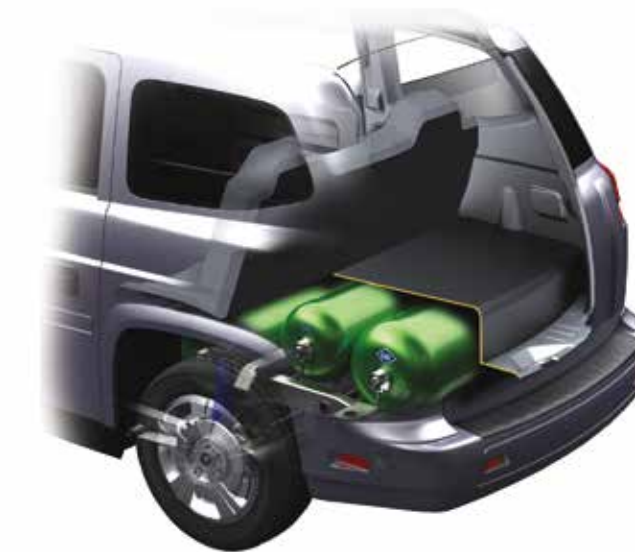
The 3-tank CNG fuel system is integrated seamlessly into the vehicle, still allowing for nearly 30 cubic feet of cargo space.
