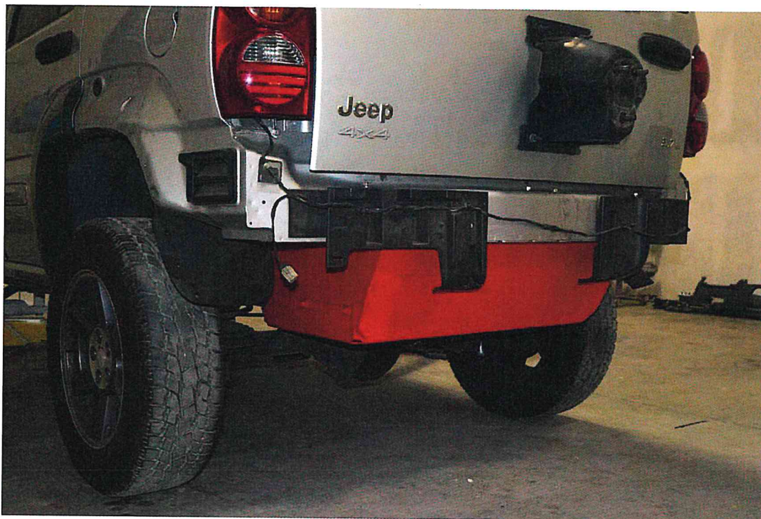
FIGURE 59. 2003 Jeep Liberty with Fuel Tank and FTEP Re-Installed
