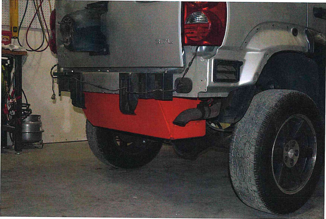
FIGURE 61. 2003 Jeep Liberty with Fuel Tank and FTEP Re-Installed
