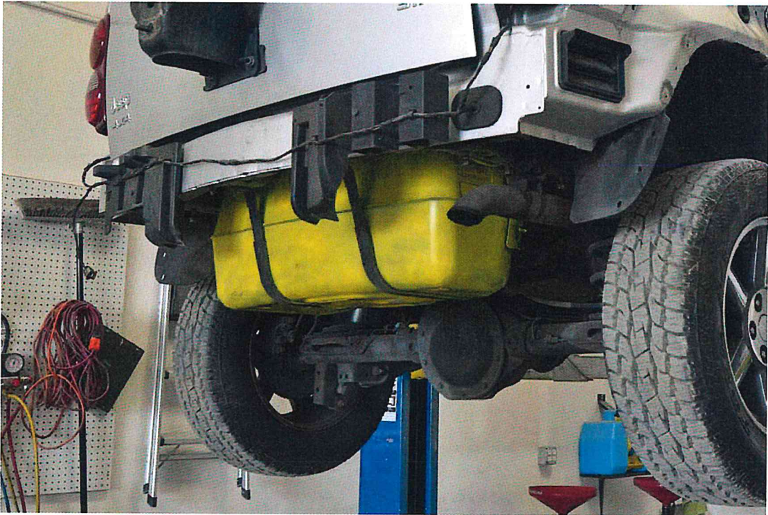
FIGURE 29. 2003 Jeep Liberty with Fuel Tank Reinstalled
