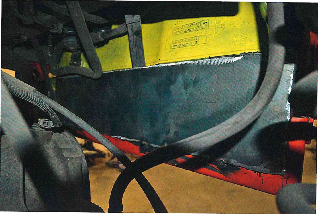
FIGURE 66. 2003 Jeep Liberty with Fuel Tank and FTEP Re-Installed
