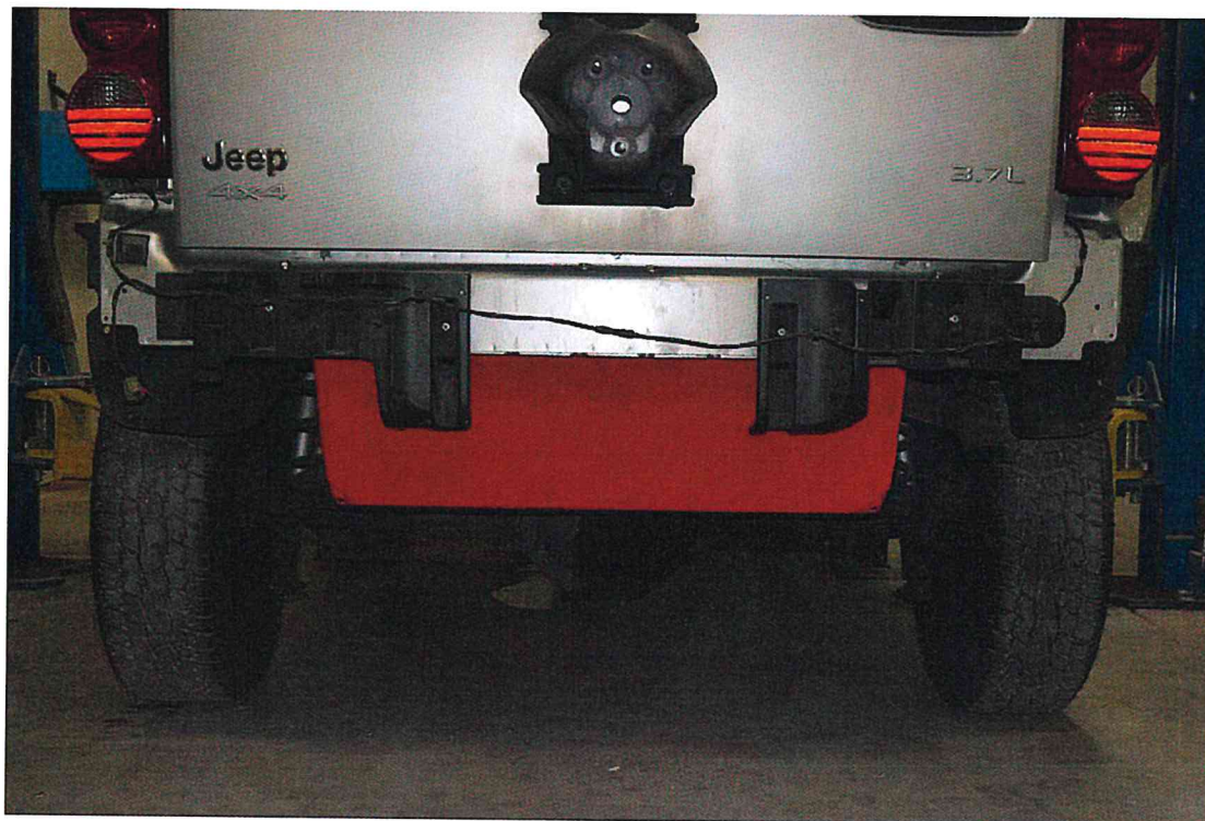
FIGURE 60. 2003 Jeep Liberty with Fuel Tank and FTEP Re-Installed
