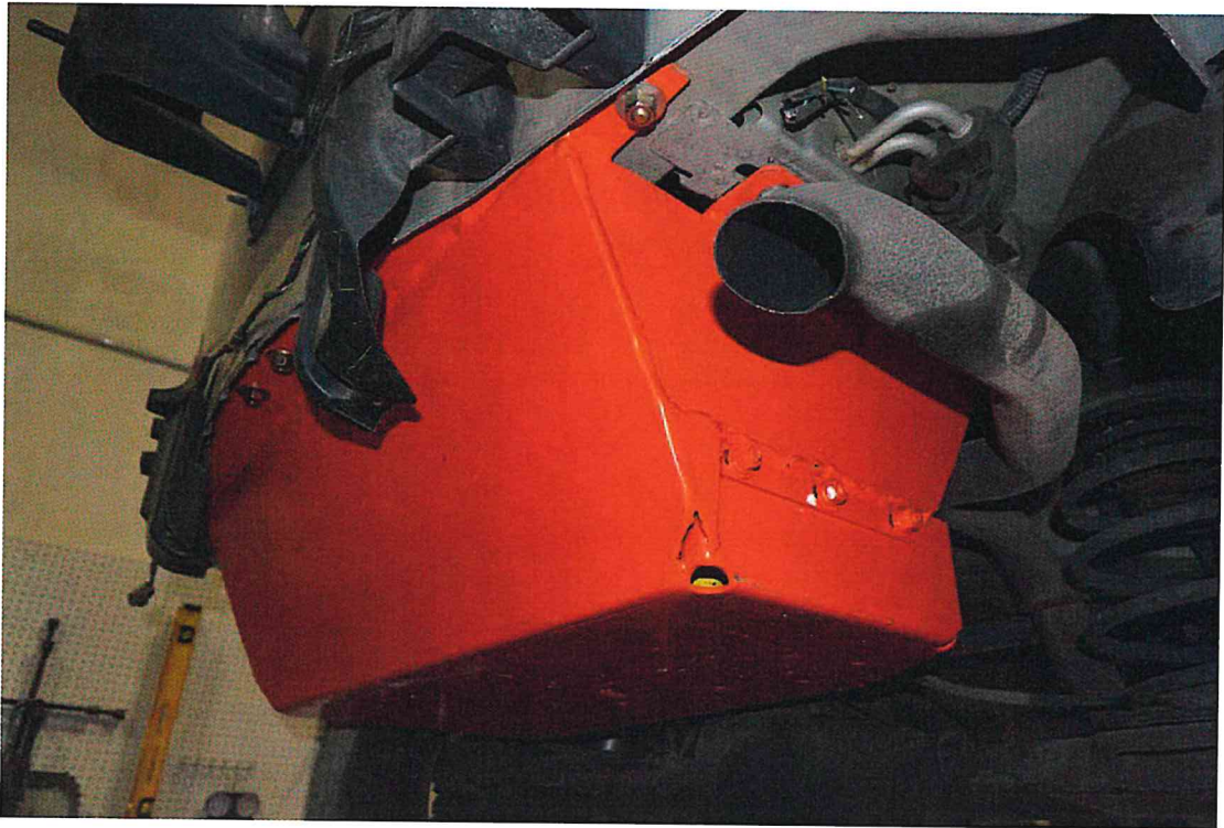
FIGURE 64. 2003 Jeep Liberty with Fuel Tank and FTEP Re-Installed
