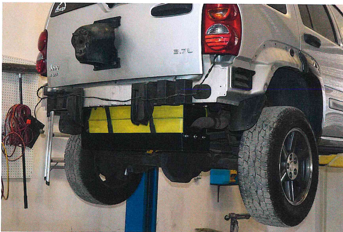
FIGURE 35. 2003 Jeep Liberty with SFK Manufacturing Model JP-4002 Skid Plate Installed
