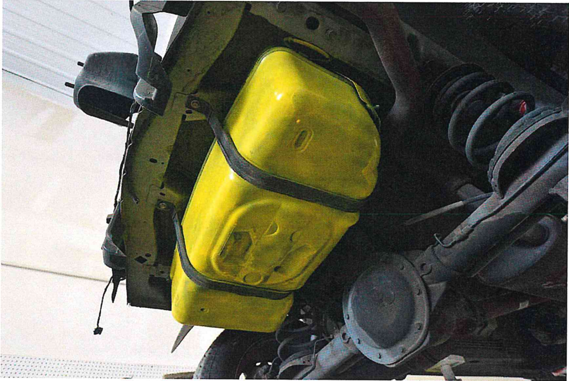
FIGURE 32. 2003 Jeep Liberty with Fuel Tank Reinstalled
