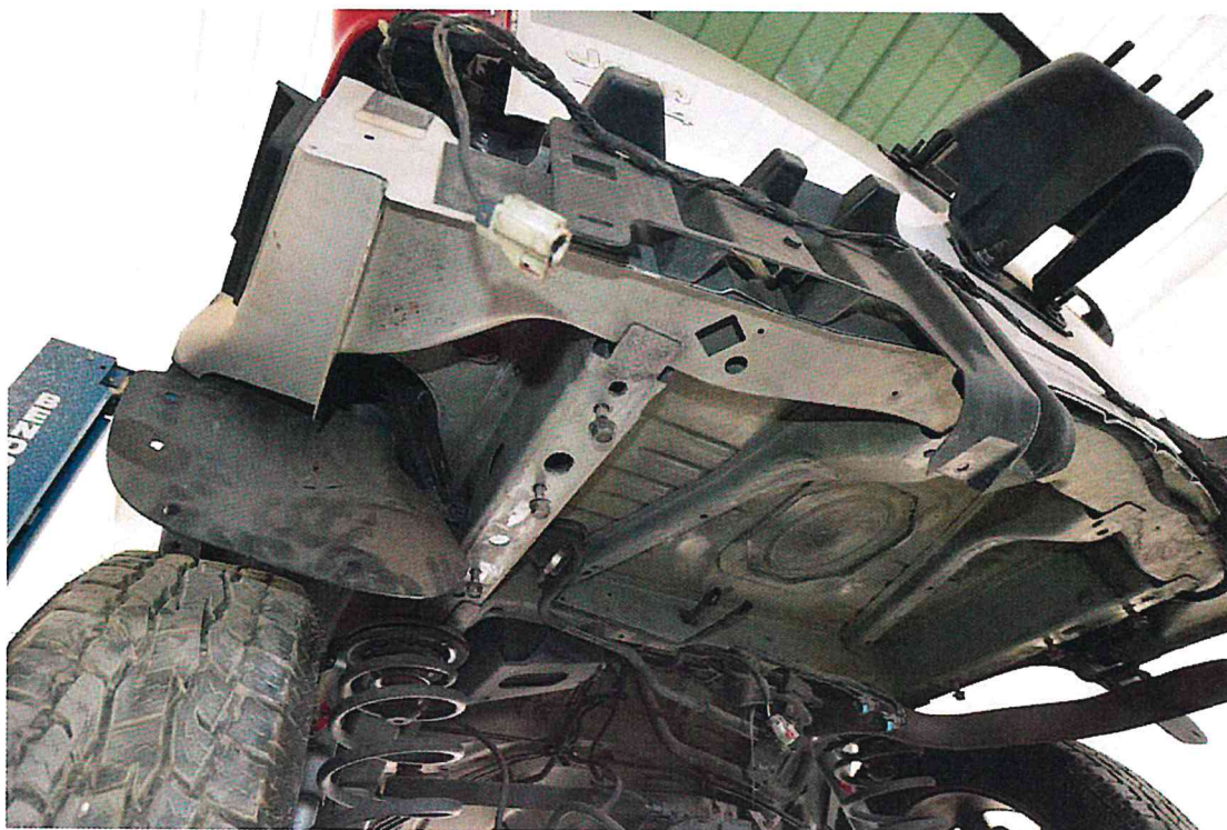
FIGURE 24. 2003 Jeep Liberty Fuel Tank Removed
