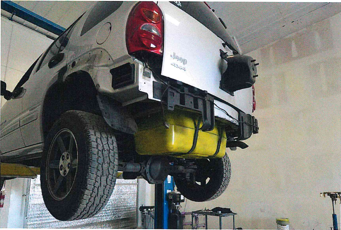
FIGURE 27. 2003 Jeep Liberty with Fuel Tank Reinstalled
