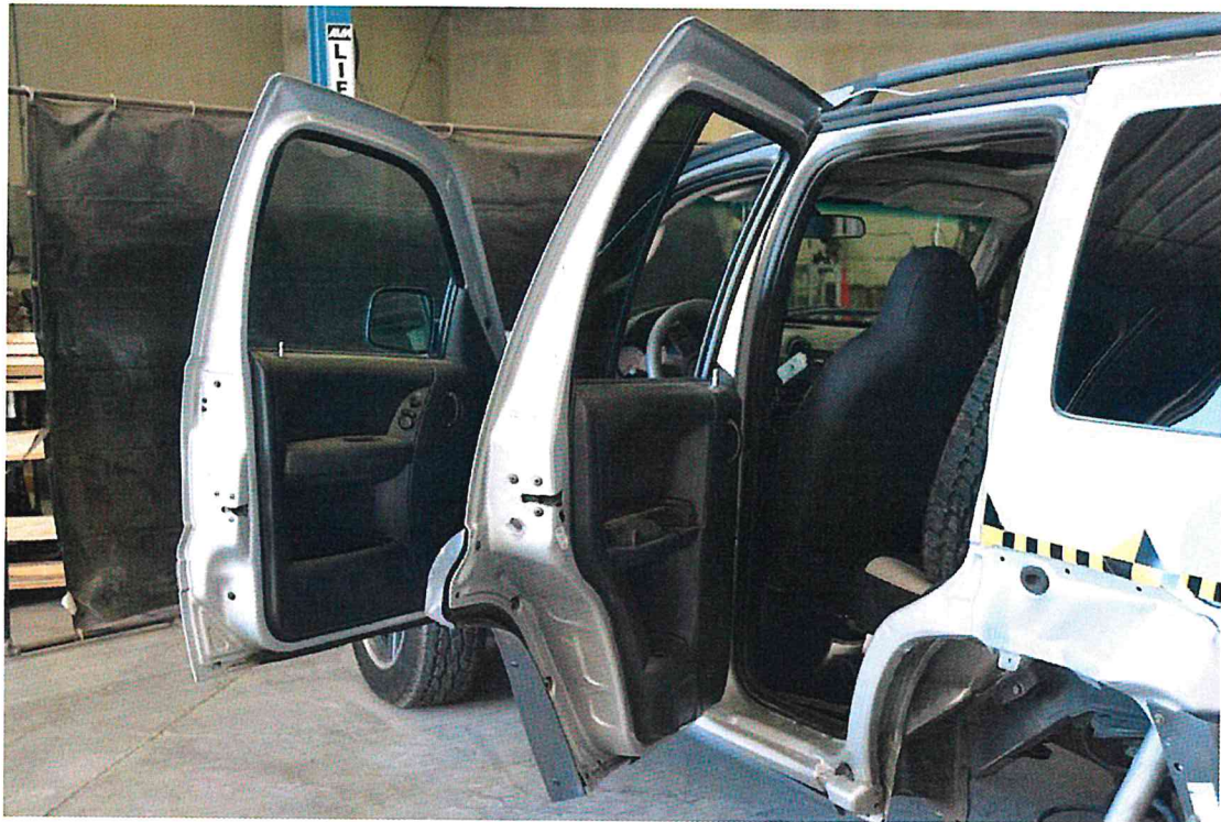
FIGURE 148. Post-Test Door Opening
