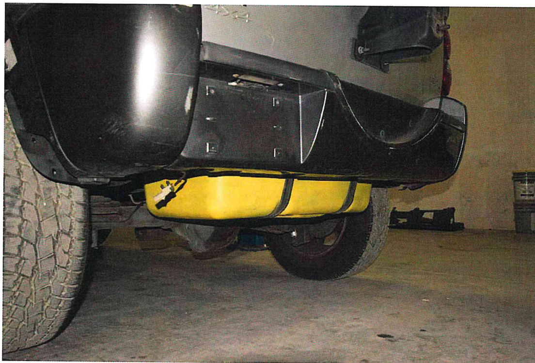
FIGURE 58. 2003 Jeep Liberty with Fuel Tank Re-Installed
