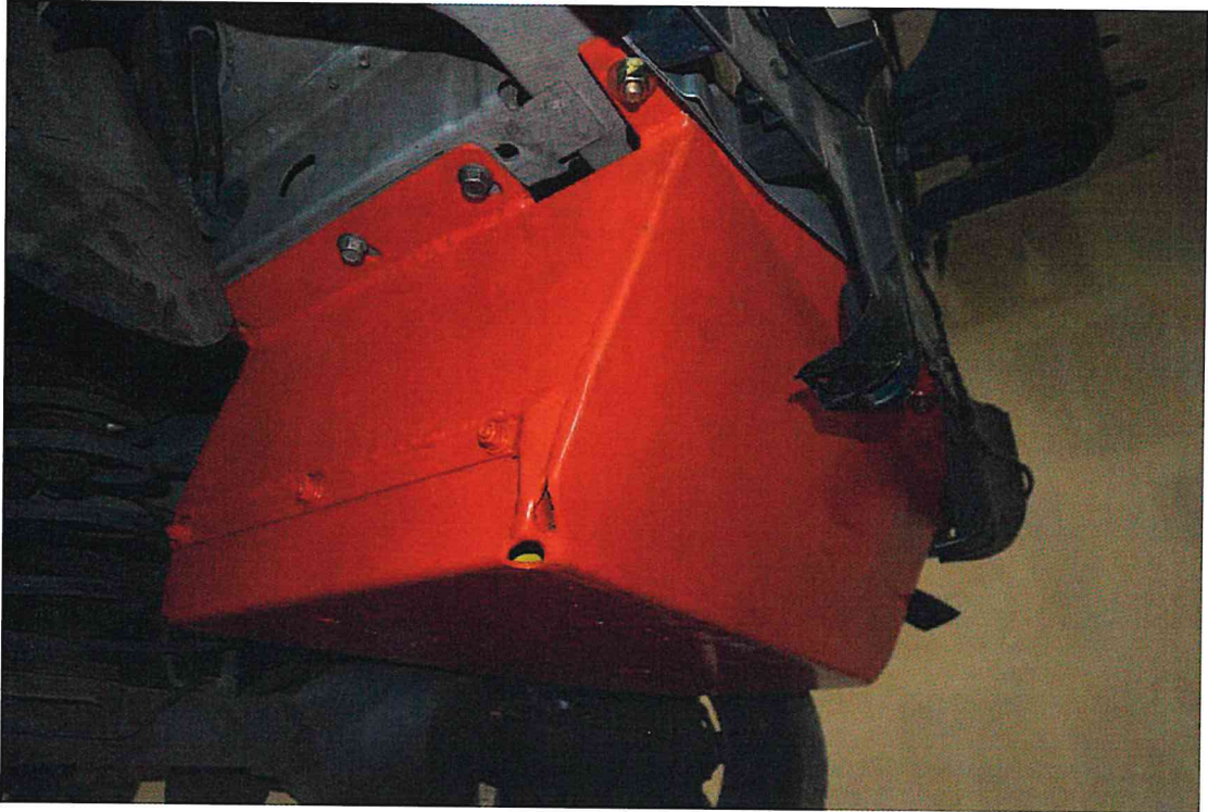
FIGURE 62. 2003 Jeep Liberty with Fuel Tank and FTEP Re-Installed
