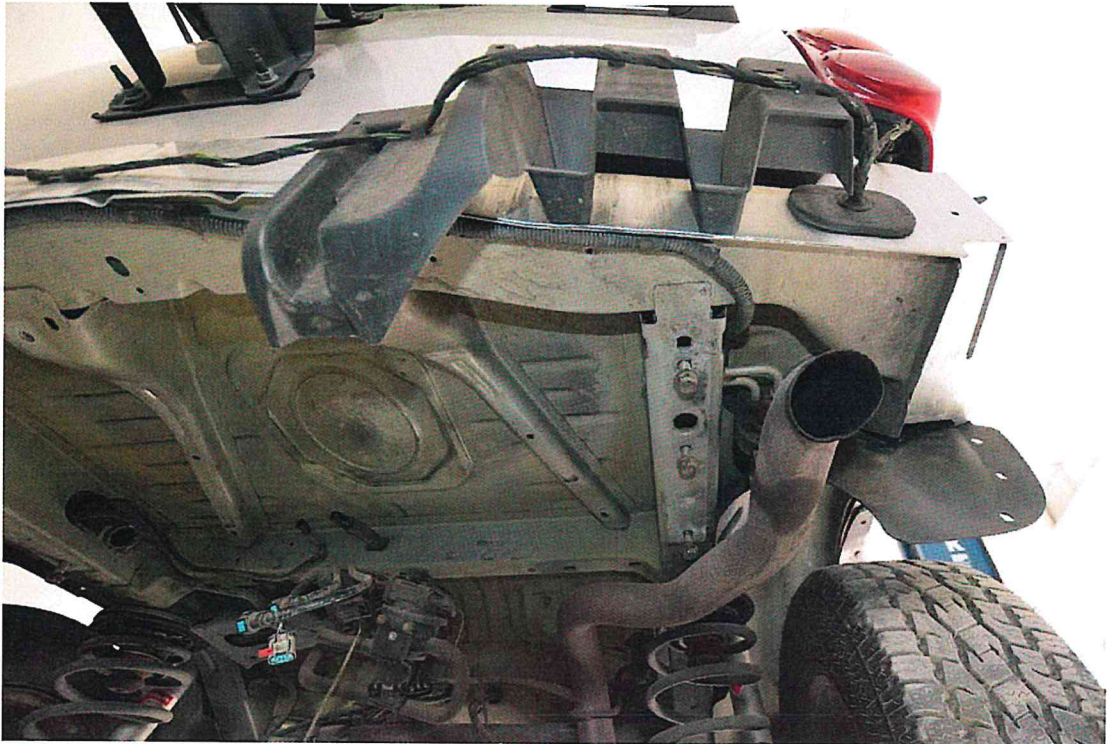
FIGURE 26. 2003 Jeep Liberty Fuel Tank Removed
