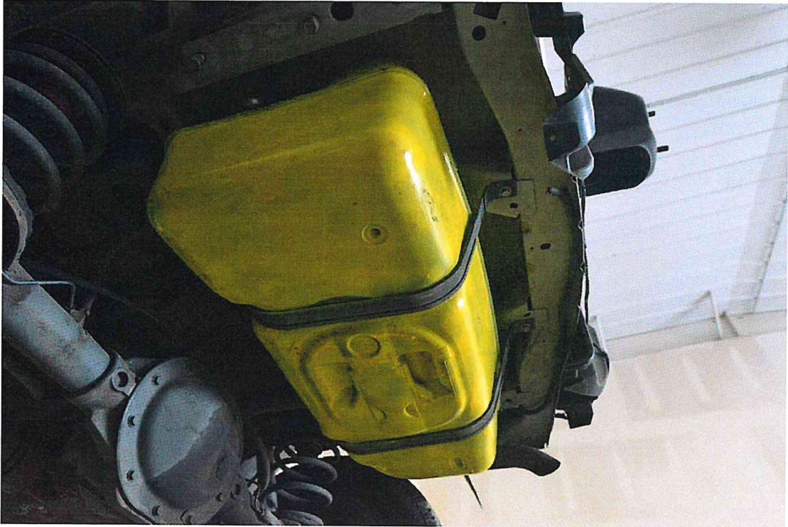
FIGURE 30. 2003 Jeep Liberty with Fuel Tank Reinstalled
