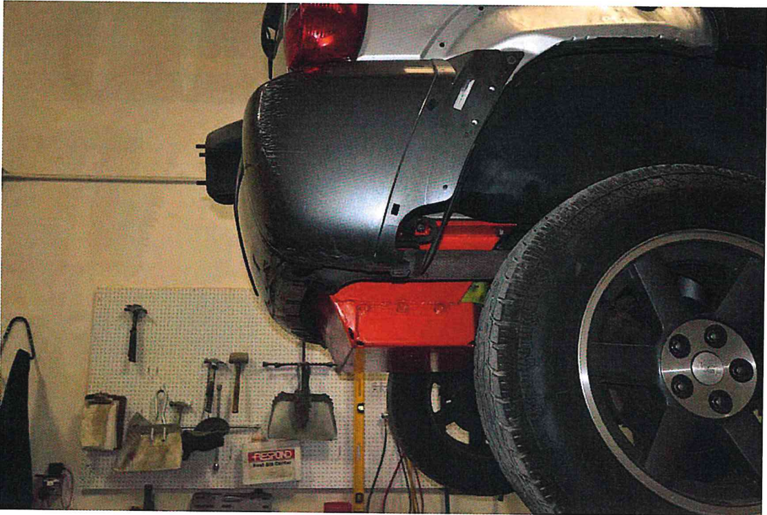
FIGURE 112. Pre-Test Fuel Tank Inspection
