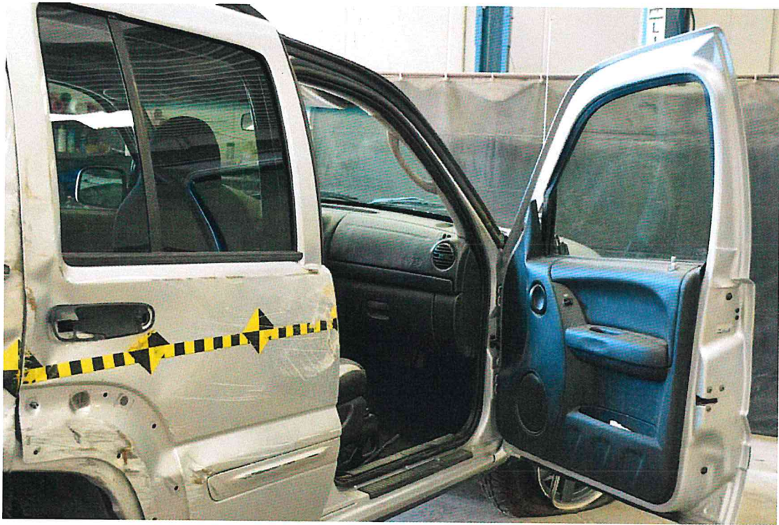
FIGURE 149. Post-Test Door Opening
